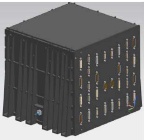
Thruster Control Unit
